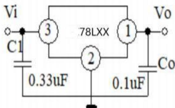
Note 1: To specify an output voltage, substitute voltage value for "xx".
